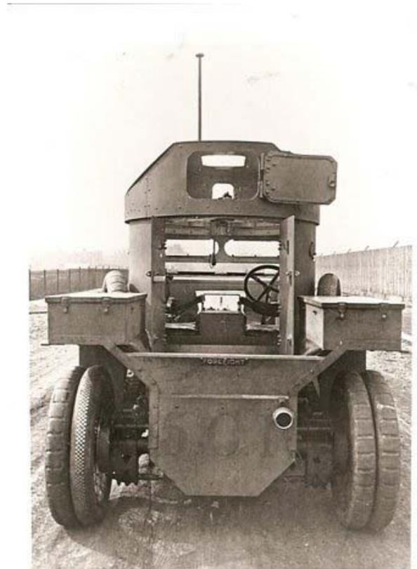
Rear view, Note interior, steering wheel, flag pole and both ordinary grooved tyres and the smooth anti skid tyres.
